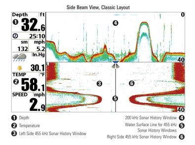
**Slanted layout:** This layout presents the two 455 kHz side sonar beams and the 200 kHz down-looking sonar beam as three panels of historical data. This layout is presented as three slanted panels. New information appears on the right and scrolls to the left.
